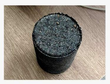
Metal briquettes are compacted blocks made from metal chips or shavings using a metal briquetting press. They reduce volume, improve melting, save resources, and enhance overall safety of a workplace.
