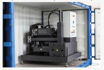
MBP Includes integrated oil collection pads. Does not include packing table — only briquette guides. Comes with see through bunker doors & oil heating elements as standard. Machines are controlled by quality Siemens KTP-400 touchscreens.
