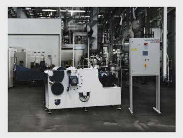
**Versatile Solution:** Single rotor shredders excel in shredding a wide range of materials including wood, rubber, plastic, paper, light metals, and general waste, even medical waste. Their adaptability suits woodworking companies seeking efficient waste management.
