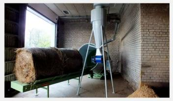
Integrated Conveyor: The integrated 4000 mm conveyor ensures smooth and continuous material handling, significantly enhancing productivity in your shredding operations. You just need to load conveyor with bales and SS-D180 does the rest.
