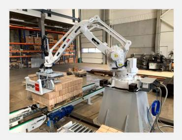
The APS-4 automates the packing process by transporting briquettes from presses to the packing machine and shrink-wrapping them automatically. It can also include automatic palletising and is designed for scalability, allowing future upgrades.
