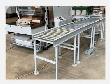
The SAPS requires manual loading of briquettes and packs them into selected thickness shrink film. It features a two-sided seam system for better dust resistance and can be used for a variety of products such as bottles and sugar packets.
