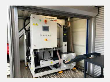
The BP-500 hydraulic press from UMP Technika is a machine that transforms sawdust into briquettes, turning unwanted waste into profits for your business. All you need is dry sawdust and electricity.
