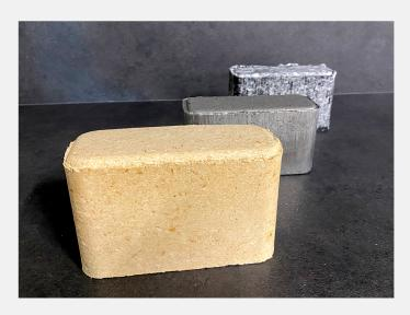
Sawdust briquettes are a clean biofuel made without any additives which are used in boilers, stoves and fireplaces. It takes about 7m<sup>3</sup> of sawdust to create 1m<sup>3</sup> of briquettes which also simplifies handling and storage.
