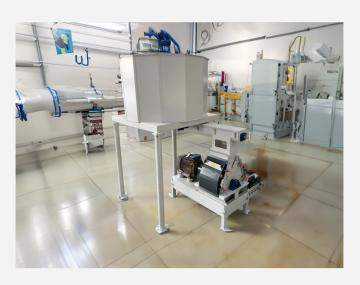
**Optimal efficiency:** The MMB-2000 configuration includes a ~2.9m3 buffer and an auger. This auger automatically doses material into the hammer mill based on its current load, optimizing energy efficiency and throughput to the next level, ensuring consistent operation, reducing downtime.
